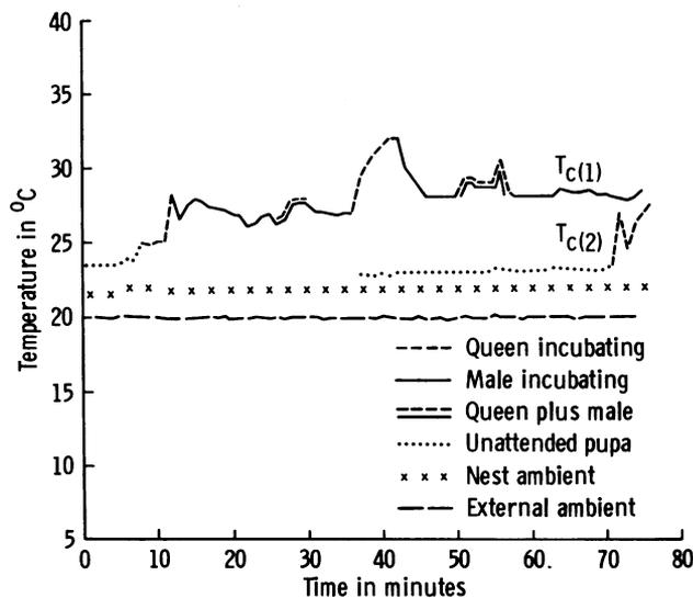
FIG. 2. Nest and pupal temperatures in a nest of *B. griseocollis* at an ambient temperature of  $20^\circ\text{C}$ . Temperatures were recorded from four thermocouples: one recorded external ambient [ $t_{A(\text{ext})}$ ]; one recorded the internal ambient of the nest [ $t_{A(\text{int})}$ ]; the others measured the temperature of two different pupae,  $t_{C(1)}$  and  $t_{C(2)}$ .
