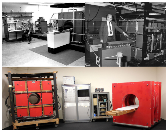
Figure 2: Paul Lauterbur and his first magnet at UIUC, 'Big Red'. Top left and right: Paul demonstrating the use of magnet in his MRI instrument. Bottom: Unboxed 'Big Red' in the new museum at the Beckman Institute, University of Illinois at Urbana-Champaign. < https://beckman.illinois.edu/visit/explore-beckman/illinois-mri-exhibit >
