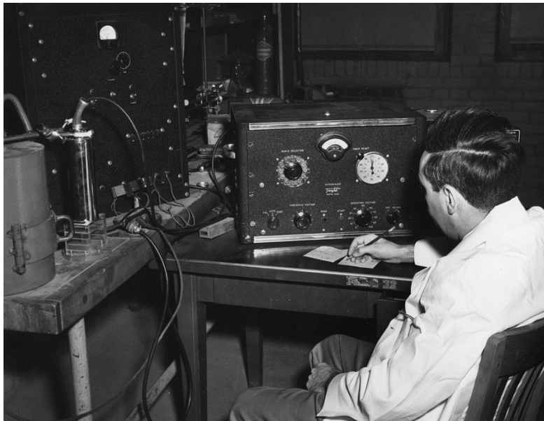
Figure 3. Martin Kamen (then associate professor of chemistry at Washington University and chemist at the Mallinckrodt Institute) sitting in front of an instrument to record radioactivity from various materials. At the extreme left is a lead-shielded container (~600 lb) in which radioisotopes were delivered from Oak Ridge, Tennessee. Also seen are various types of Geiger counters to record the presence of radioactive materials. (Photo taken in 1950; courtesy of Washington University Photographic Services Collection, Washington University Libraries, Department of Special Collections)
