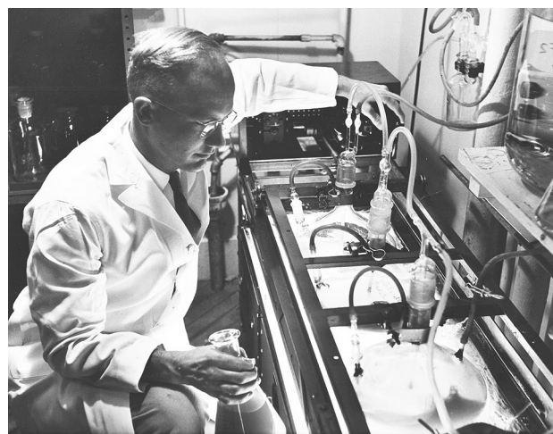
Fig. 2 Andrew A. Benson with his microalgal culture system. Pure cultures of Chlorella or Scenedesmus were grown in illuminated Fernbach flasks. After reaching a high cell density, cell suspensions were transferred to a lollipop for irradiation. From the private collection of Dee Benson
