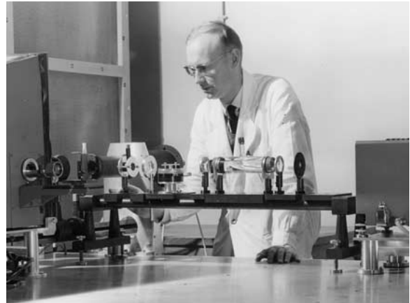
Figure 4. Paul Mathis (author). Top: 7 April 1994; bottom: working on his first flash absorption apparatus in March 1966.
