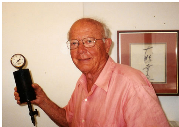
Fig. 8 Andy Benson holding an aspirator, with a vacuum gauge at the top; this instrument was used by Martin Kamen during 1940s and he used this to aspirate reactive gases. Photo, 2001. Source: Govindjee
