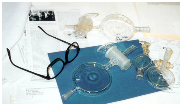
Fig. 6 A photograph of several glass “lollipops” used for putting algal suspensions to which ^{14}\text{CO}_2 was injected and then after illumination, the suspension was let out, by opening the stopcock, into boiling methanol. Photo, 2001. Source: Govindjee
