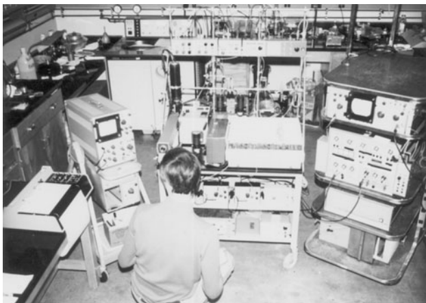
Fig. 6 The instrument room, in early 1974, in the laboratory of Warren L. Butler (1925–1984) at the University of California San Diego, California. It shows an instrument setup that was filled with oscilloscopes, chart recorders and photomultipliers. The instruments, shown here, were built and used by one of the authors (Reto J. Strasser; in the foreground). Specifically, the system had low voltage home-made oxygen monitors with amplifiers and external offset boxes to measure high amplification of O_2 in the zero to 8.0 ppm range, a 12-bit data acquisition with ms time resolution and two analog channels, analog and digital signal visualization, floppy disk drive, power supply, a tower with an oscilloscope for fast recording by single shot and polaroid photography, three pen recorders to monitor electric stabilities, fastest available X–Y recorder, available at that time, monochromators for excitation and emission spectra and photomultiplier tubes (EMI and Hamamatsu) with four high voltage supplies. From data, obtained with such instruments, Strasser and Butler evolved models of excitation energy distribution and redistribution in photosynthesis (see e.g., Butler and Strasser 1977). Source Photo was taken by an unnamed assistant in Butler's lab
