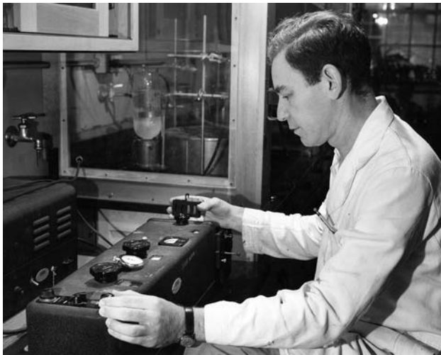
Fig. 8 Martin Gibbs using a battery powered hand-operated Beckman DU Spectrophotometer, ~1950 at the Brookhaven Lab. Photo courtesy of the Brookhaven National Laboratory
