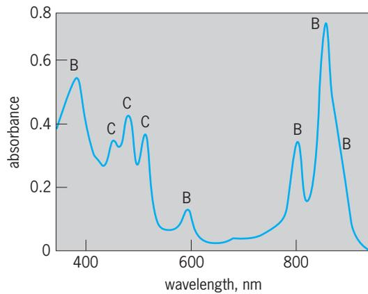
Fig. 14. Absorption spectrum of chromatophores from the bacterium *Rhodospirillum rubrum*. Absorption bands attributed to BChl *a* are labeled as B, and those attributed to carotenoids as C. (After R. K. Clayton, *Photosynthesis: Physical Mechanisms and Chemical Patterns*, Cambridge University Press, 1981)
