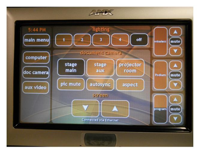
Same middle screens as the computer selection. The Document camera is in the drawer on the right side of the large podium. Currently we are using an Elmo with extending camera boom and side lights. The small monitor on the tray can be used to see alignment.
