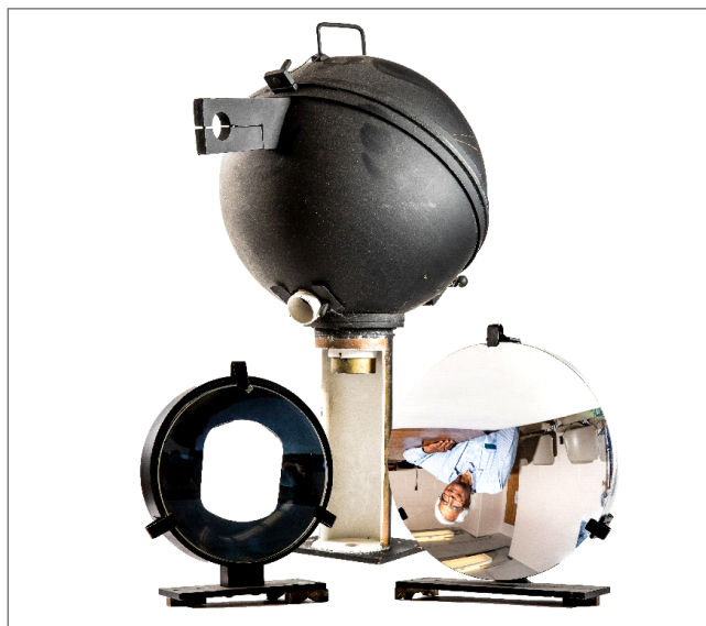
Figure 10: From left, a lens, an integrating sphere, and a mirror were used in early photosynthesis experiments. Photo by Fred Zwicky
