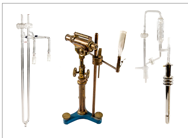
Figure 2: A manometer, left; a telescope and a capillary tube, center; and a distillation column that were used in his early photosynthesis experiments. Photo by Fred Zwicky
