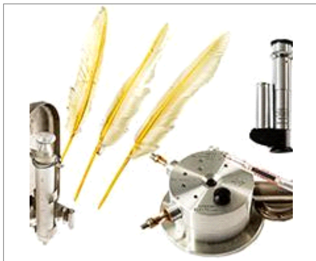
Figure 8: From left, a syringe for transferring precise quantities of algal cells, feathers used to dust glass vessels, an electrometer to measure low light intensities, and a hand-held spectroscope for checking the spectral distribution of light in photosynthesis experiments. Photo by Fred Zwicky
