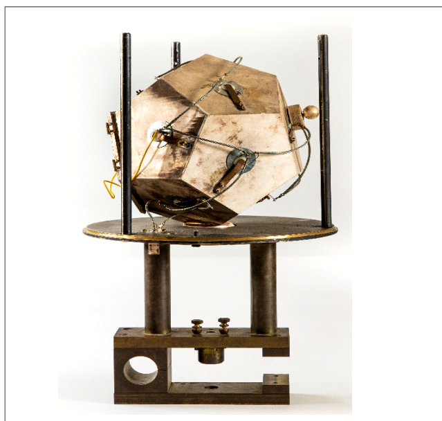
Figure 3: Govindjee’s former graduate student Carl Cederstrand built this dodecahedron with 12 photocells. With this instrument, they demonstrated the physical presence of different spectral forms of chlorophyll a . Govindjee had earlier determined that the different spectral forms of chlorophyll a must contribute to different photochemical reactions in photosynthesis. [See Laura Cederstrand and G. Govindjee (2022) Carl Nelson Cederstrand (1927-2022): A biophysicist, an innovator, and a wonderful person. International Journal of Life Sciences 11(1): 21-27] Photo by Fred Zwicky
