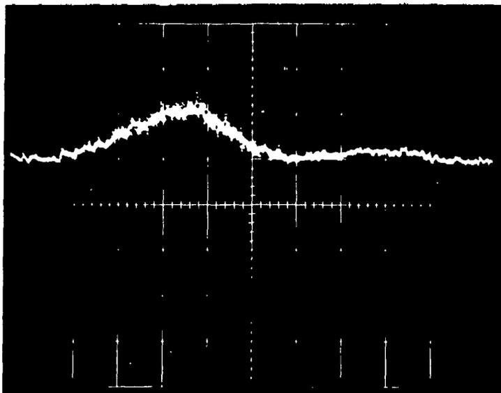
Figure 14. A photograph of a sampling oscilloscope trace showing a mode-locked laser pulse as monitored by a photomultiplier. Horizontal scale is one nsec/division.
