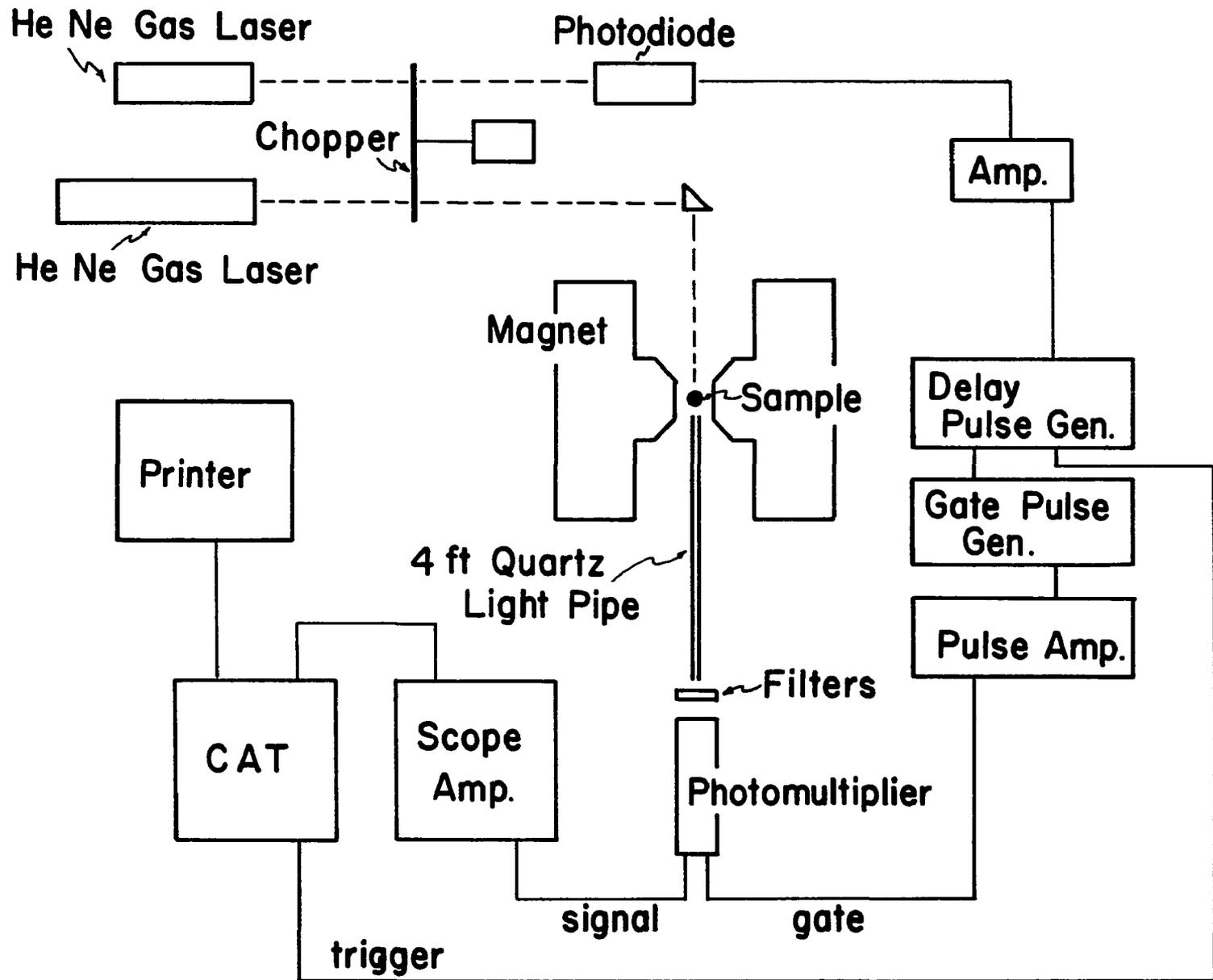
identical to the gate pulse generator. A variable delay was provided by triggering the gate pulse generator with the second spike of the differentiated output of the delay pulse generator. The delay was adjusted so that the gate pulse generator was turned on in 0.1 milliseconds after the incident beam which excites the sample was cut off.
