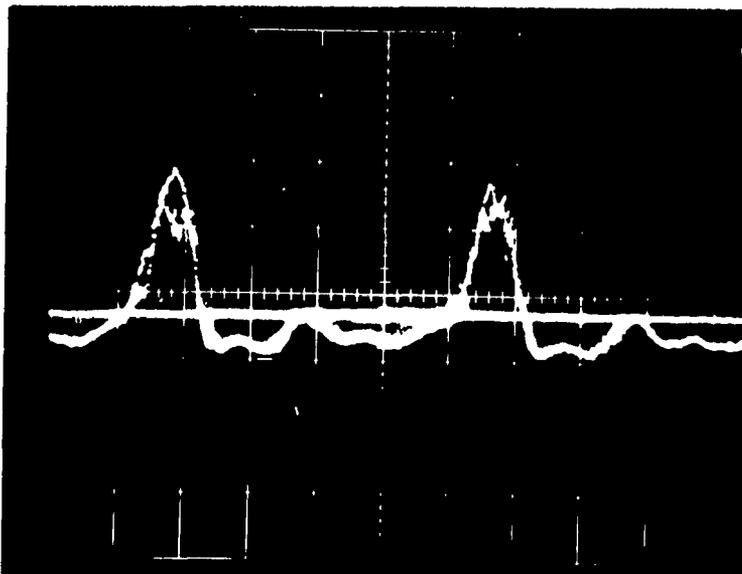
Figure 5. A photograph of a sampling oscilloscope trace showing a mode-locked laser pulse as monitored by a "PIN" diode. Horizontal scale is two nsec/division.
