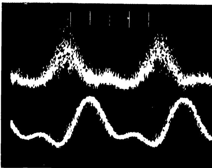
Figure 23. A photograph of a sampling oscilloscope trace showing the mode-locked laser pulse as monitored by the measuring photomultiplier (top curve); and as monitored by the trigger photomultiplier (bottom curve). Horizontal scale is two nsec/division.
