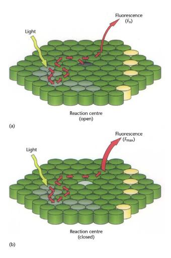
**Figure 5** Schematic drawing showing excitation energy transfer from one chlorophyll molecule to another in the antenna system. Green cylinders represent chlorophylls *a* and *b*, and yellow cylinders represent carotenoids; the dark cylinder in (a) represents an open reaction centre and the grey cylinder in (b) represents a closed reaction centre.
