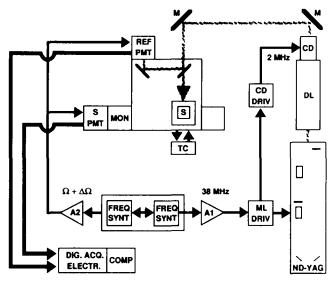
Fig. 2. A block diagram of the instrument. ND-YAG, Neodymium-Yttrium-Aluminum Garnet laser; DL, dye laser; CD, cavity dumper; M, Mirror; CD Driv, CD driver; ML Driv, mode-locker driver; A1, A2 amplifiers; TC, temperature controller;  $\Omega$ , chosen frequency (multiples of 2 MHz;  $\Omega$ , 40 Hz cross correlation signal; Freq synt, frequency synthesizer; Mon, monochromator; S, sample; PMT, photomultiplier; Comp, computer; Dig. Acq. Electr., digital acquisition electronics. (See text.)
