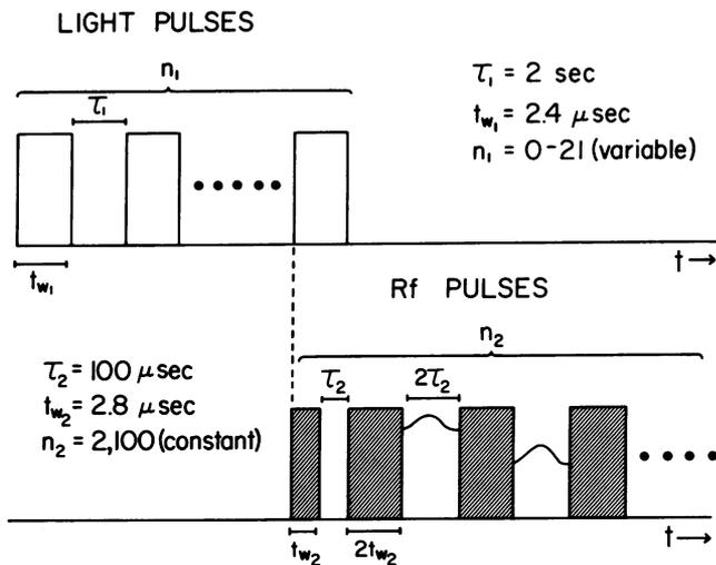
FIG. 1. Experimental procedure used to measure  $1/T_2$  after a sequence of light pulses.  $1/T_2$  is the decay rate for the exponential decrease of the proton spin echoes in the Carr-Purcell rf pulse sequence.
