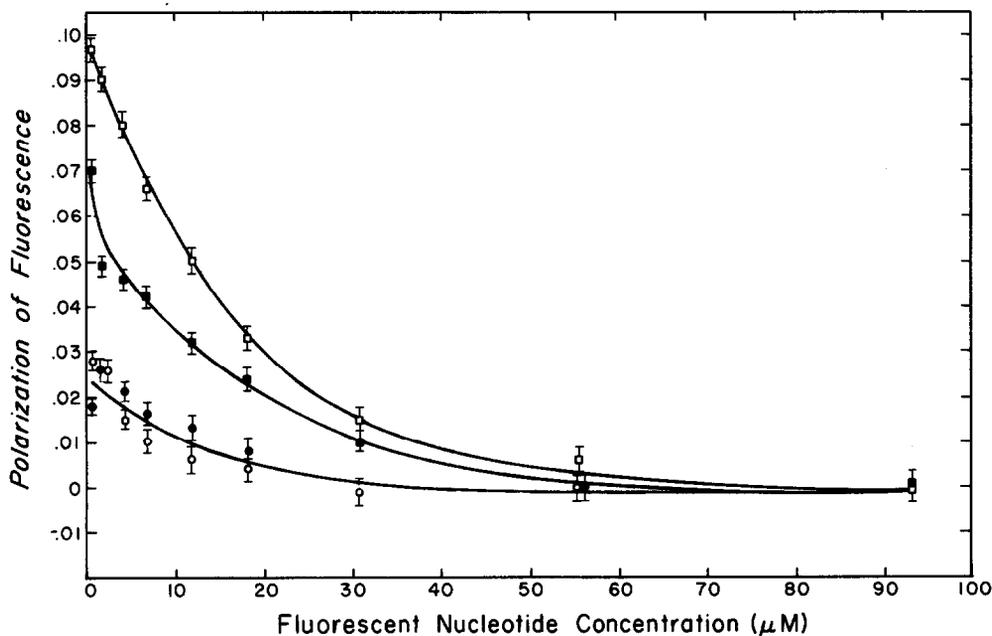
Fig.2. Degree of polarization of  $\epsilon$ -adenine fluorescence as a function of concentration of adenine analogs.  $CF_1$  protein was buffered at pH 8 in 25 mM Tricine-NaOH, plus 5 mM  $MgCl_2$  and 500  $\mu M$   $NaH_2PO_4$  (closed symbols) or 5 mM  $MgCl_2$  only (open symbols).  $[CF_1]$  was  $\sim 4 \times 10^{-6}$  M ( $\epsilon$ ATP data, circles) and  $\sim 5 \times 10^{-6}$  M ( $\epsilon$ ADP data, square). Error bars represent approximate contribution of instrument fluctuation.
