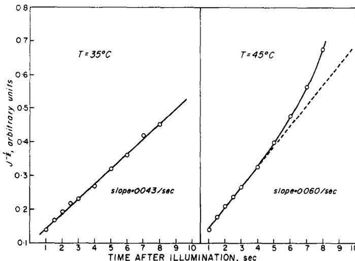
Fig. 8. Decay curves of  $J^{-1/2}$  for DCMU treated *Synechococcus* at 35 and 45°C. The decay is still linear at 35°C but deviates from linearity at temperatures of 45°C and higher.
