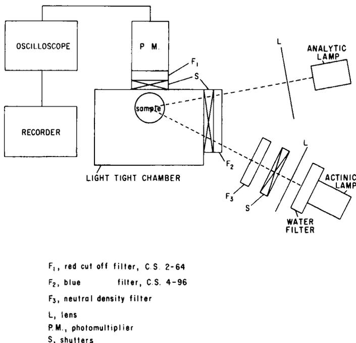
Fig. 1. Diagram of the experimental apparatus for measuring delayed light emission (DLE), temperature-jump delayed light emission (TDLE) and chlorophyll fluorescence yield.
