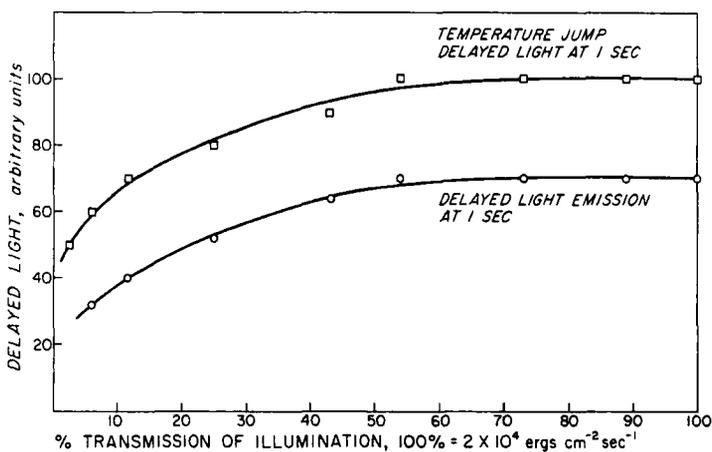
Fig. 2. Light curves for both DLE and TDLE. Saturation occurs for both at about  $1.1 \times 10^4$  ergs  $\text{cm}^{-2} \text{sec}^{-1}$ .
