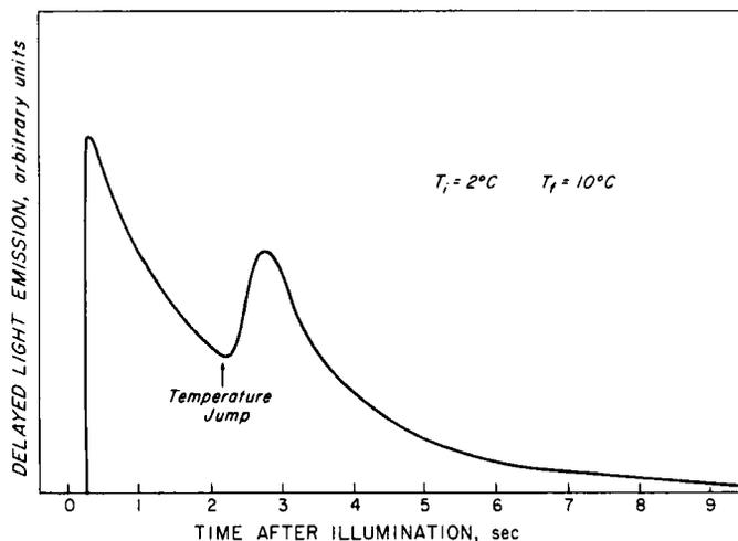
Fig. 10. Chart trace of DLE and TDLE: A temperature jump from 2 to 10°C; other details as in Fig. 9.
