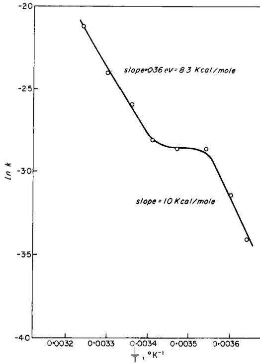
Fig. 12. Arrhenius plot of the back reaction constant of  $Z^+$  and  $Q^-$  in *Chlorella*. The section of zero slope occurs in the (physiological) temperature range of  $10^\circ\text{C} \rightarrow 20^\circ\text{C}$ . The slopes of the curves differ slightly for temperatures above and below the zero slope temperature range.
