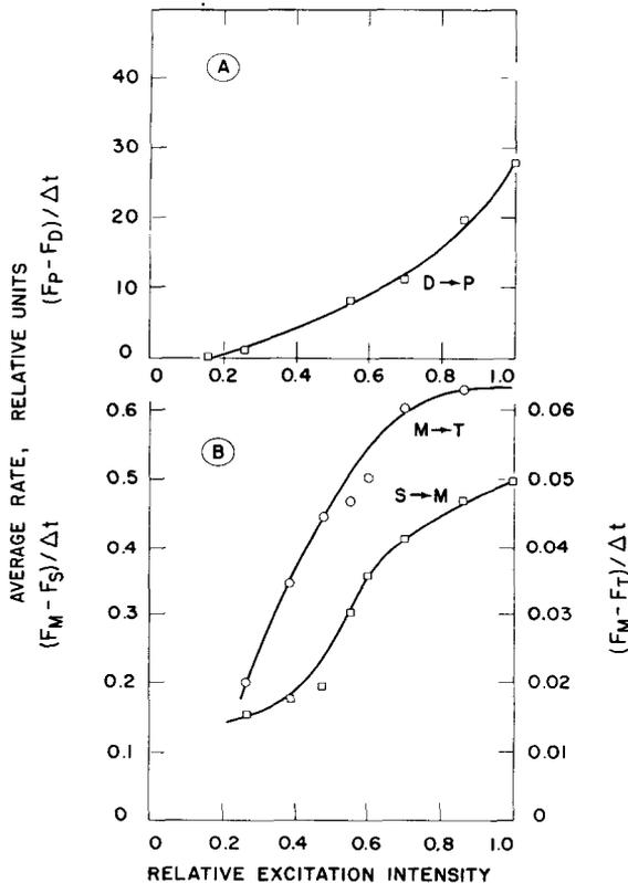
Fig. 6. Average rate of change in the fluorescence yield as a function of the intensity of exciting light. (A): For *DP* rise; (B) for *SM* rise, and *MT* decline; intensity  $1.0 = 9.2 \times 10^3$  ergs  $\text{cm}^{-2} \text{sec}^{-1}$ ; all other conditions same as in Fig. 1(B).
