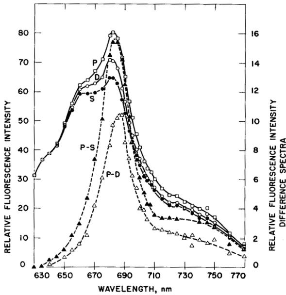
Fig. 8. Fluorescence emission spectra at the stage *D* (open circles), *P* (open squares), and *S* (solid circles). Difference spectra *P-D* (open triangles) and *P-S* (solid triangles) on an expanded (5X) ordinate scale. Details as in Fig. 1(B) with the exception that C.S. 2-58 was used instead of C.S. 2-64 filter.
