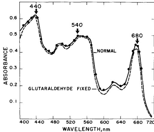
Fig. 11. Absorption spectra for normal (solid) and fixed (dashed) cells adjusted at the red peak. Fixation was in 3% (v/v) glutaraldehyde (see text for details); buffer, 0.05 *M* potassium phosphate plus 0.25 *M* NaCl.
