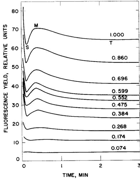
Fig. 4. Slow transient of the fluorescence yield of Chl *a* at different intensities of excitation. Intensity 1.000 =  $9.2 \times 10^8$  ergs  $\text{cm}^{-2} \text{sec}^{-1}$ ; other conditions as in Fig. 1(B).
