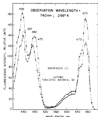
Fig. 3 (upper left). Excitation spectra of cell suspension of *Ch. pyrenoidosa* and of the aerobic sonicated material (pH 4.6) at room temperature (298 °K).  $\lambda$  observation = 740 nm.
