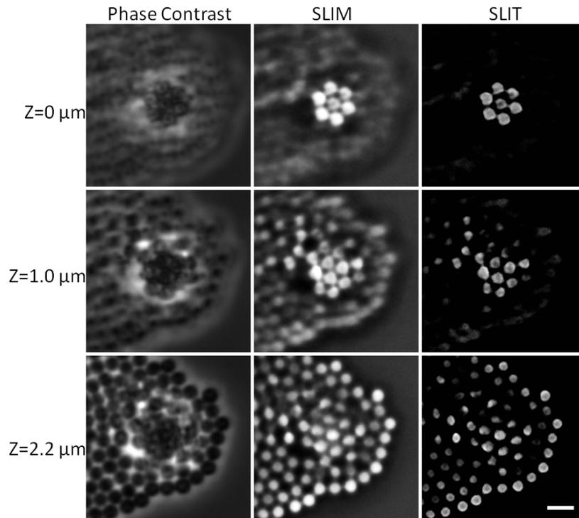
Fig. 5. Comparison of sectioning effect in phase contrast, SLIM and SLIT measurement of the same photonic crystal samples. The sample is made by 1  $\mu\text{m}$  silica beads index matched with isopropyl alcohol (IPA). Scale bar: 2  $\mu\text{m}$ . Objective: Zeiss Plan-Apochromat 63  $\times$  /1.4 oil.
