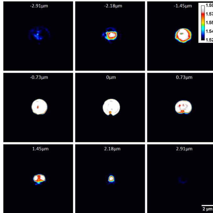
Fig. 4. Refractive index map of  $3.1\ \mu\text{m}$  polystyrene beads in immersion oil (Zeiss Immersol 518F, refractive index 1.518) at different Z positions. Objective: Zeiss Plan-Apochromatic  $63\times/1.4$  oil.
